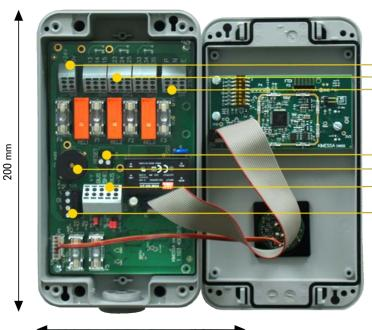
24 VDC Supply 3x pot. free relay contacts 230 VAC Supply
