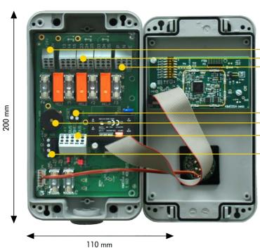
Pressure range:atmospheric ± 10%Air humidity:15...90 % R.H. non-condensingPosition sensitivity:noneLong term output drift:< 2% signal loss/month</td>Life span at 20 °C:6-8 years, depending on the<br/>application
