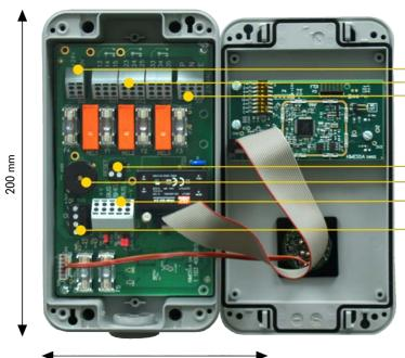
24 VDC Supply 3x pot. free relay contacts 230 VAC Supply
