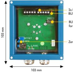
2x BUS-Connectors BUS-End-Resistor
